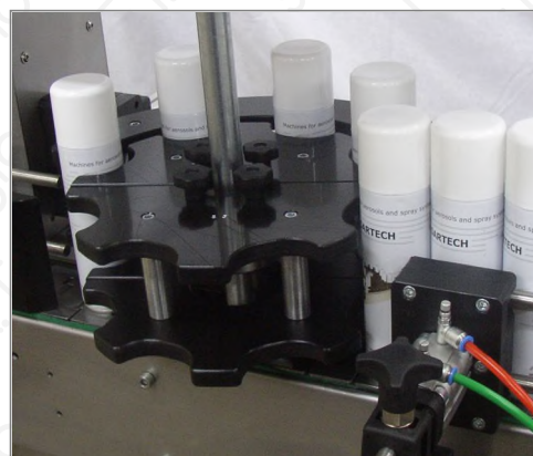
Rotational mechanism is a checkweigher DWR/H series
